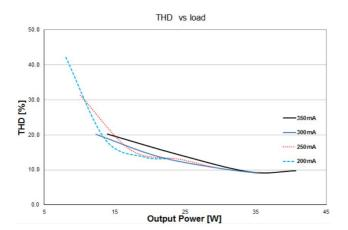
Typical THD vs load of EM FIT 40W 350 D CS L G2
