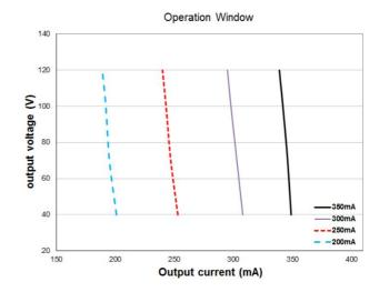
Typical Operating window of EM FIT 40W 350 D CS L G2
