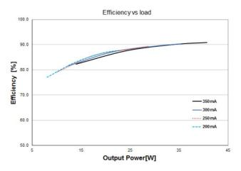
Typical Efficiency vs load of EM FIT 40W 350 D CS L G2
